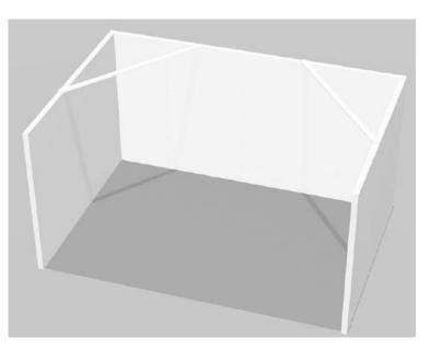
For lighting, you can order arm lights from the accessories page or to place track lights in the booth, order through show management. They can be hung on the angled bars provided with the Artwall package. If more lighting is required, you can order a 2"x4"x15' wood beam that will affix to the front of the booth.
